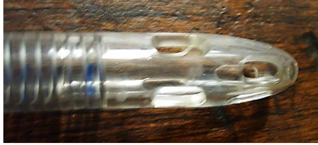
FIGURE 35 – ‘Open’ tip design that includes an open orifice with 8 sideholes displayed the best flow characteristics from the three designs studied in static loop testing.
